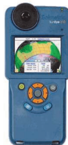
Fig. 3.1. Solmetric Sun Eye Device. Source: Solmetric
