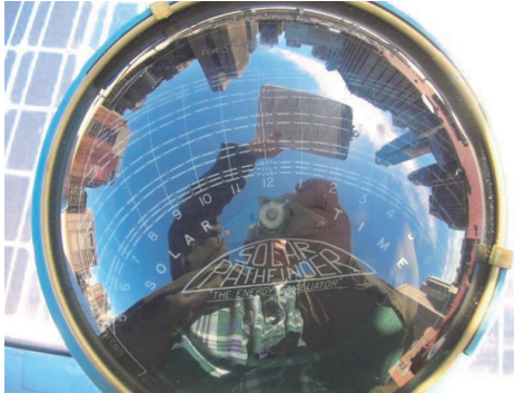
Fig. 3.2 Solar Pathfinder On-Site Close-Up – objects shading the site are reflected in dome of device)
